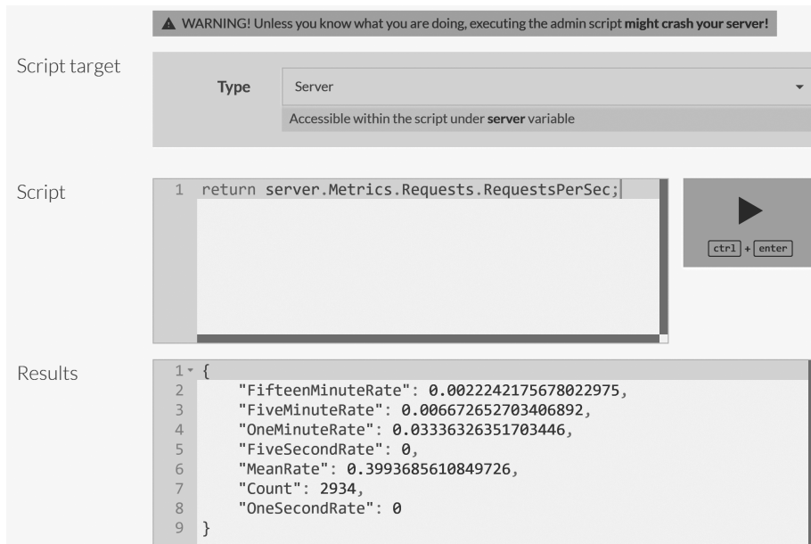
Figure 16.10: The Admin JS Console lets you run scripts against the current server instance.
