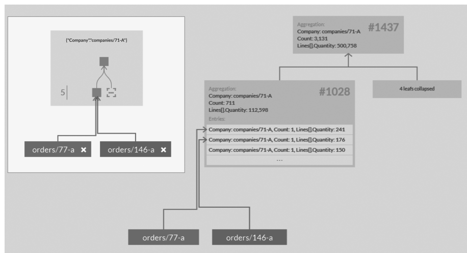
Figure 11.7: MapReduce works as a tree once we have enough entries for a particular value
